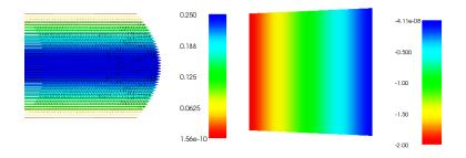
**Figure:** Illustration of Poiseuille flow in 2D as computed with  $P_2 - P_1$  elements in FEniCS. Left image shows the velocity vectors while the right image shows the pressure. Both velocity and pressure are correct up to round-off error.
