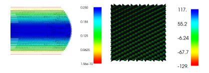
**Figure:** Illustration of Poiseuille flow in 2D as computed with  $P_1 - P_1$  elements in FEniCS. Left image shows the velocity vectors while the right image shows the pressure. The velocity is correct but the pressure is *not*. The  $P_1 - P_1$  discretization violates the inf-sup condition.
