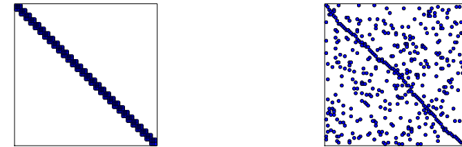
Fig. 4.21 Matrix sparsity pattern for left-to-right numbering (left) and random numbering (right) of nodes in P3 elements.
