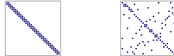
Fig. 4.20 Matrix sparsity pattern for left-to-right numbering (left) and random numbering (right) of nodes in P1 elements.
